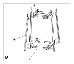
Use the Screws (1) pre-assembled in their respective eyelets to connect Upper Supports (3) to the Lower Supports (1) and to fix the Emitter Screen between the Upper Supports.
