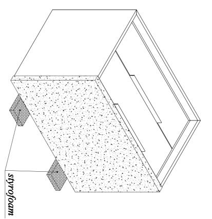
Caution: when attaching the legs, please do not put the cabinet directly on floor to avoid damaging the concrete top. Please put the cabinet gently on the styrofoam to protect the tabletop while attaching the legs.
