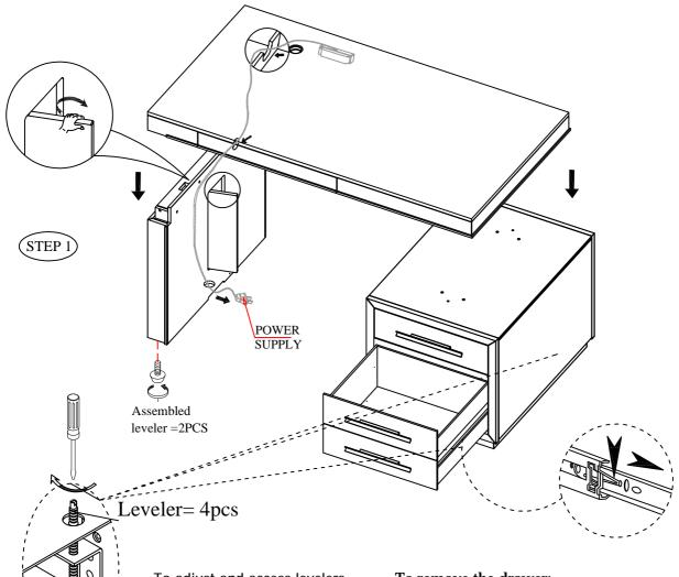
To adjust and access levelers, first remove plastic cap if it have with a flat-head screwdriver. Using the same screwdriver, proceed to turn leveler clockwise to raise the piece, or counterclockwise to lower the piece.
