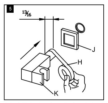
5. Apply Teflon tape (H) to the threaded end, the fix the cover plate (J) onto the wall supply holder (K) and screw the wall supply holder (K) into the hand shower outlet.
