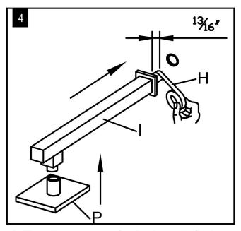
4. Turn the water on for 1 minute to flush any debris. Apply Teflon tape (H) to the threaded tail pipe and install the shower arm (I) into the outlet on the wall, Then connect the top shower (P) to the spout.
