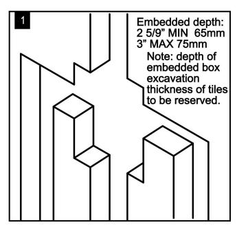
1. According to the site condition and the installation size requirement and to make a hole, the hold size is 180mm(length)X130mm (width)X65~75mm(deep).
