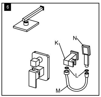
6. Add rubber washers (L) at both ends of the shower hose (M). Connect shower hose (M) to the wall supply holder (K) and hand shower (N). Then, place the hand shower (N) to the wall supply holder (K).
