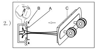
Step.2: Wire fixture to wires in outlet box. Black wire is positive, white is neutral, Copper wire is for Ground. Attach Fixture (C) to mounting hardware (A) using screws (B) to secure.
