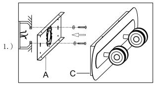
Step.1: Remove mounting hardware (A) from Fixture (C) and install to electrical box.
