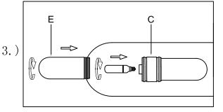
Step.3: Install 40 Watt candelabra base bulb. Then, Thread glass (D) into fixture (C).
