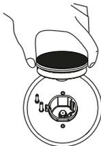
3. Remove the natural gas orifices with a 9/32" (7 mm) nut driver.
