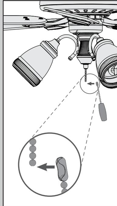
Connect the pull chain pendants to the short chains coming from the switch housing.
