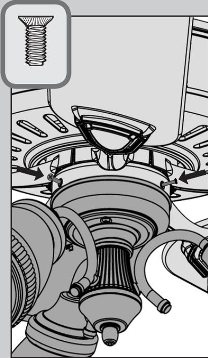
Install the three switch housing screws, found in the
