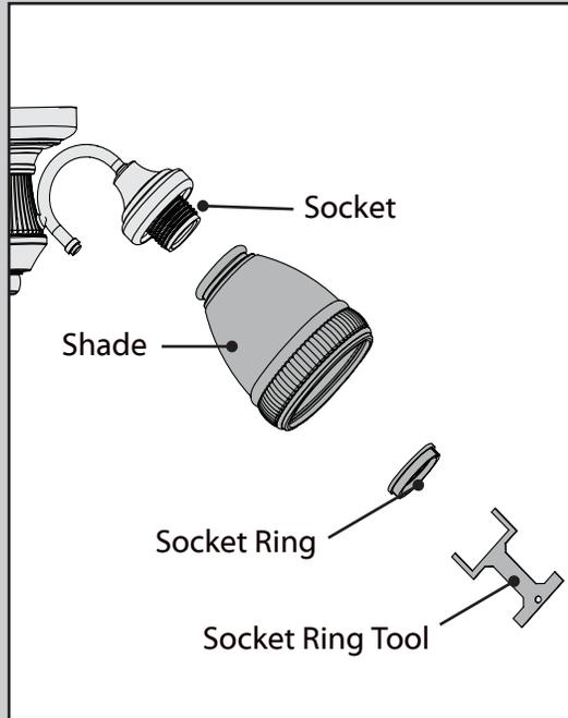
Remove the socket rings from the sockets.
