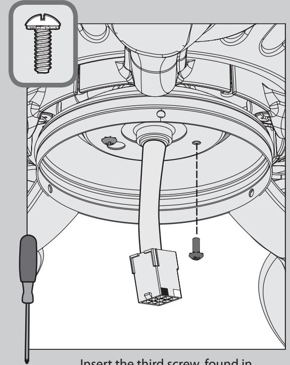
⊗ Insert the third screw, found in the
