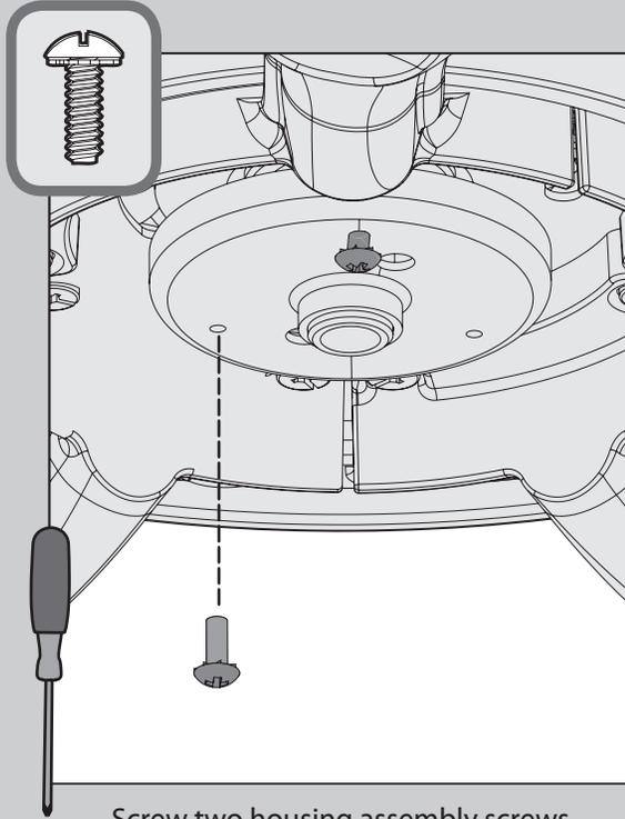
⊗ Screw two housing assembly screws from the
