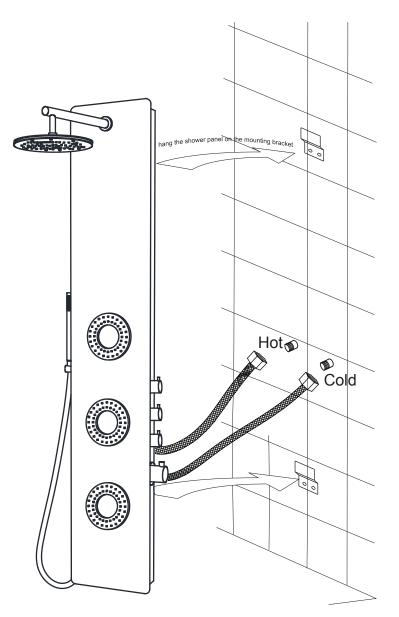
**Step 4A** Screw the cold and hot water hose from the shower panel to the supply lines in the wall.
