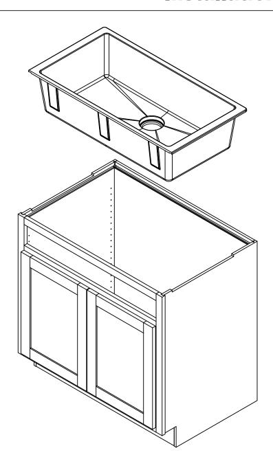
NOTE: If Undermount Sink is installed in its minimum (36 inches) recommended cabinet, side clips are not required as sink can rest on cabinet side walls.
