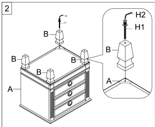
Step 2: Attach 4 legs (B) with cabinet (A). Using allen key (H2) to lock with 4\*bolts (H1)
