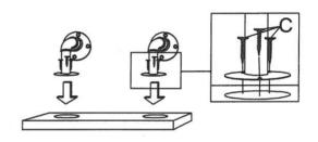
Step3: Stick the flange(part 3)to the wall mounting and mark 4 holes location of flange with marker
