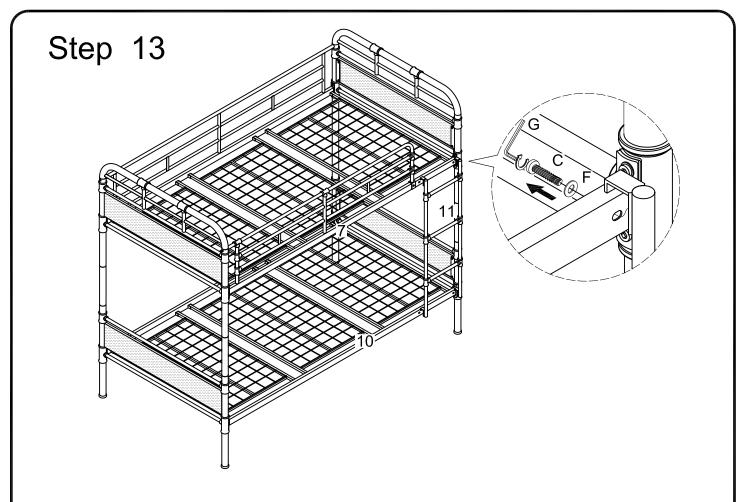
Loosen and remove the ladder (11) from the bed frame.
