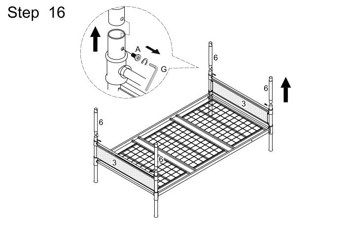
Lift and separate the bunks and the support posts (6).
