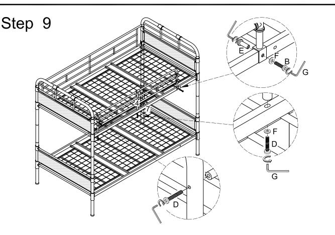
Secure parts together using the hardware as shown in the diagram. Tighten securely with wrench (G).
