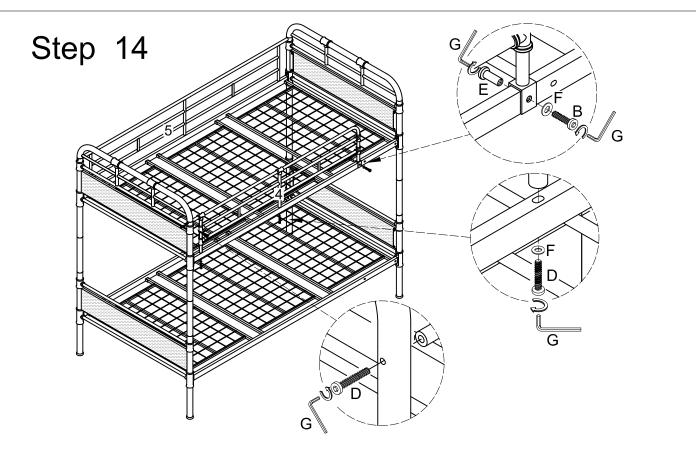
Loosen and remove the open guardrail (4,5) from the bed frame.
