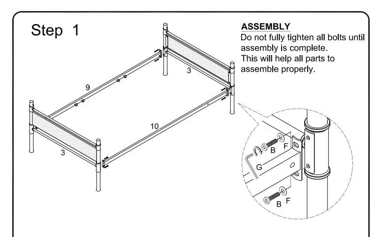
Secure parts together using the hardware as shown in the diagram. Tighten securely with wrench (G).
