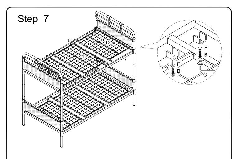
Secure bed supports (12) as shown in the diagram. Tighten securely with wrench (G).
