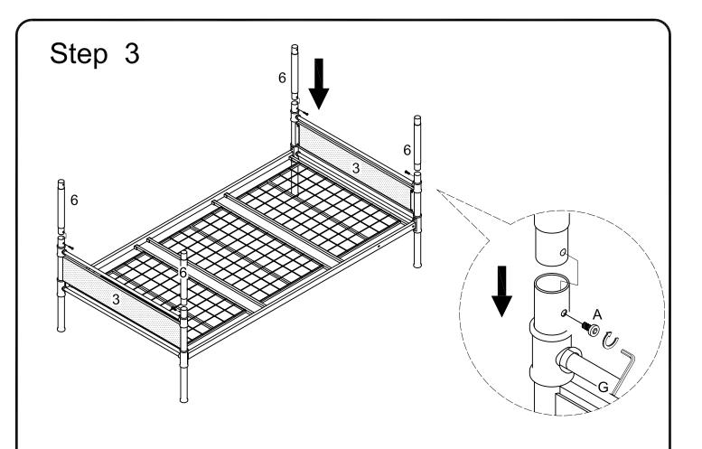
Place support legs (6) and secure with hardware as shown. Tighten securely with wrench (G).
