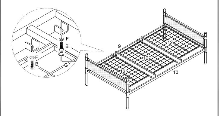
Secure bed supports (12) as shown in the diagram. Tighten securely with wrench (G).
