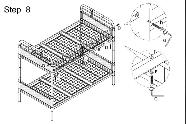
Secure parts together using the hardware as shown in the diagram. Tighten securely with wrench (G).
