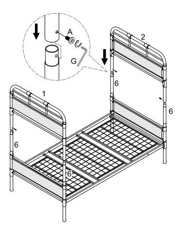
Place parts (1) and (2) and secure with hardware as shown. Tighten securely with wrench (G).
