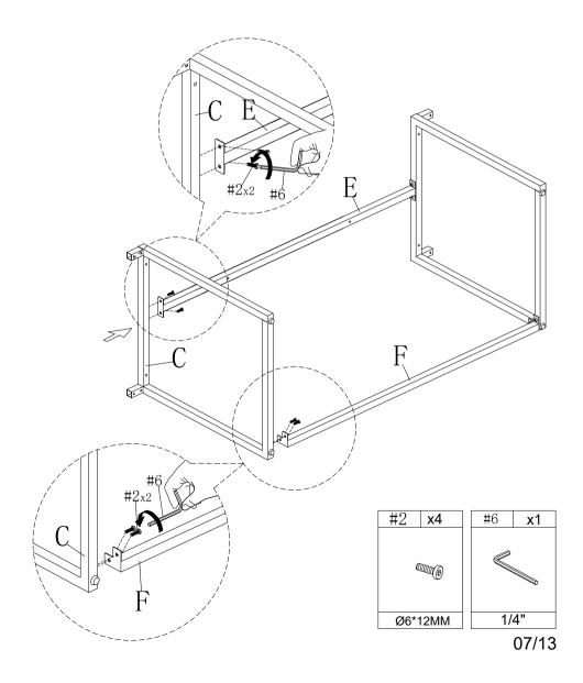
1.Use bolt #2 to connect part B with part (C&D) .tighten screw #2 with allen key #6.
