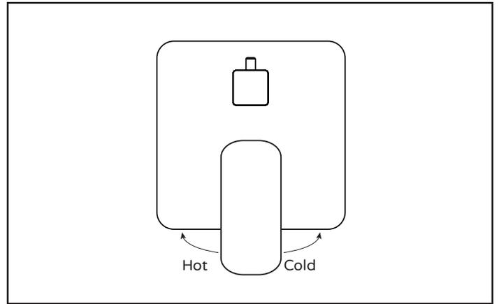
While ON, turn valve handle to the left for HOT and right for COLD.
