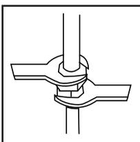
To prevent damage to the tube body, tighten the connections by carefully using two wrenches as shown. Use caution to not bend the stem. Check for leaks.
