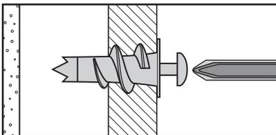
For use when attaching light loads onto plasterboard partitions.
