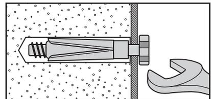
For use with heavier loads such as TV and HiFi speakers and satellite dishes etc.
