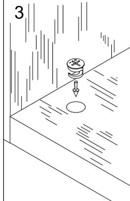
Turn the female camlock clockwise with a screwdriver.
