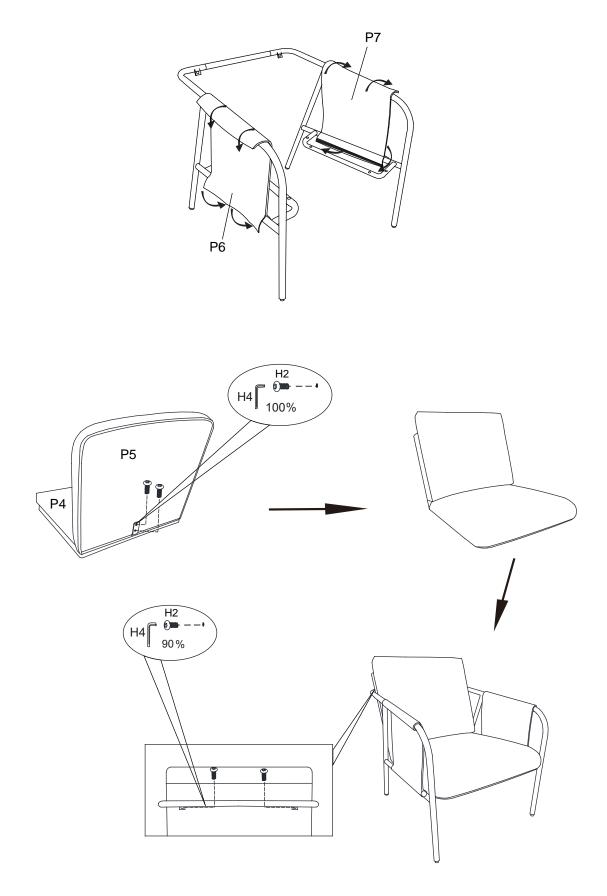
Step 3. Fix bottom of seat cushion to metal frame by using bolts (H3) and allen wrench (H4). Security tighten all bolts in step 2,3.
