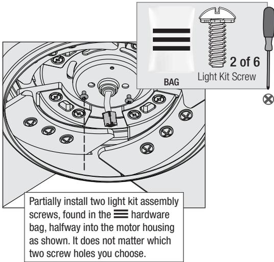
Partially install two light kit assembly screws, found in the hardware bag, halfway into the motor housing as shown. It does not matter which two screw holes you choose.
