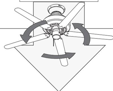
Downdraft (counterclockwise rotation) creates a direct breeze and maximum cooling effect.
