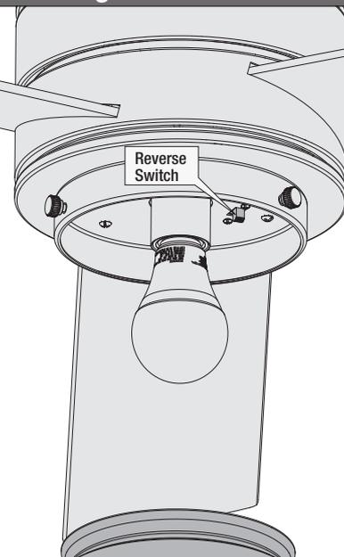
Ceiling fans work in two directions: downdraft (counterclockwise rotation) and updraft (clockwise rotation). To change the direction of air flow, turn the fan off and let it come to a complete stop. The reversing switch is located inside the light fixture. It can only be accessed when the glass is removed. Slide the reversing switch to the opposite position. Restart the fan.
