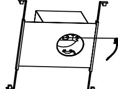
Screw adaptor into socket in recessed housing.
