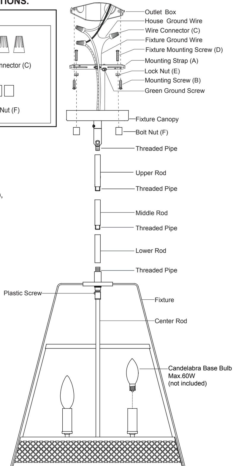
4. Pull out the source wires from the outlet box. Make wire connections using wire connectors (C) as follows:
