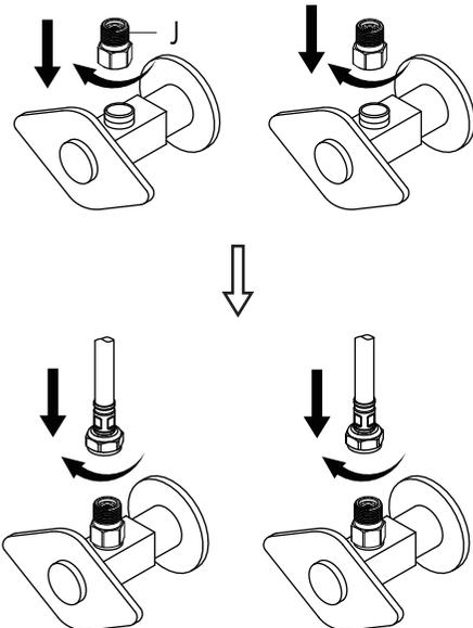
Before connecting waterlines to main valve, attach brass check valves (J) to angle stops (not included), then connect waterlines to brass check valves (J) and tighten until snug. Turn on angle stops and check for leaks (**DO NOT TURN FAUCET ON**).
