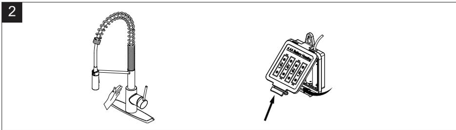
If the handle is closed, turn the handle to the on position and move your hand in the sensor area. If the sensor flashes 10 times continuously and slowly, then replace the 4 "AA" batteries.
