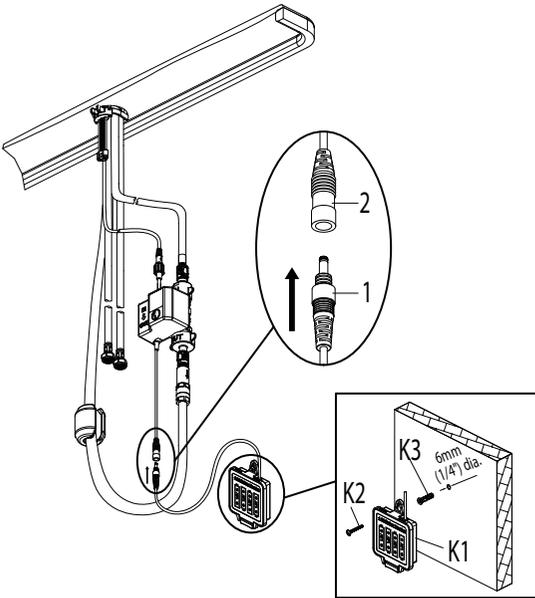
Drill a hole in the wall using a 6mm (1/4 in.) diameter drill bit. Install the battery pack (K1) using the molly anchor (K3) and screw (K2) provided. Insert the battery pack cable (1) into the control box connection (2).
