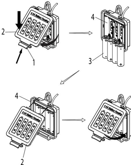
To open the battery housing, squeeze the tabs (1) on the cover (2), then remove the cover (2). Install the four AA batteries (3) included by matching the positive (+) and negative (-) ends on the battery (3) to the (+) and (-) markings in the battery pack (4). The negative ends of the battery (3) should always connect to the spring end of the battery slots in the battery pack (4). Reinstall the battery pack cover (2) by pushing up and snapping into place.
