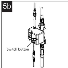
However, if you want to continue to use the faucet with the sensor feature, you need to tighten the switch button completely with a coin clockwise. At this time, you can use the faucet with the sensor feature.
