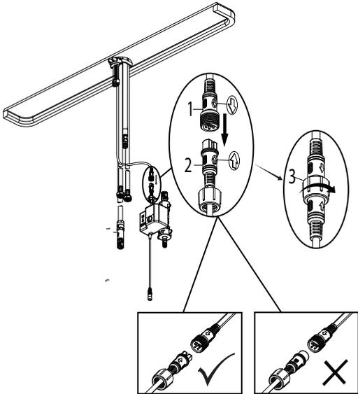
Install the data cable (1) to the control box connection (2). Ensure the arrows on the data cable and control box connection are aligned to one another to ensure proper installation. Ensure they are tightly connected by firmly pushing together. Secure the connection by hand tightening the nut (3) in a clockwise direction onto the threaded sensor cable.
