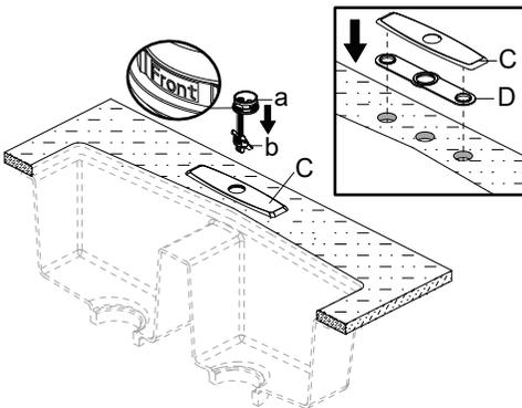
Place the escutcheon (C) and the gasket (D) on the sink. Insert the base (a) into the escutcheon (C). **NOTE:** "Front" on the base (a) must face the front of the sink. The two mounting plates (b) on the base (a) must be loose and movable during the installation of the base (a). If the sink is uneven, use silicone under the gasket (D).
