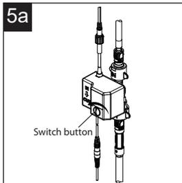
If you want to use the faucet without the sensor feature, you can loosen the switch button completely with a coin counterclockwise. At this time, you can use the sensor faucet just like a regular kitchen faucet.
