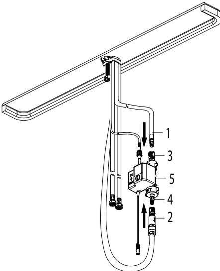
Connect the hose (1 & 2) to the connector (3 & 4) on the control box (5). Push firmly together until they snap into place.
