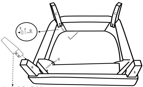
According the "Inner" Label sticker on leg, please make sure the leg bevel face is inside
