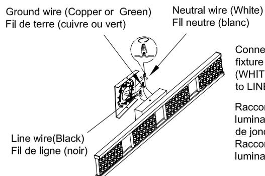
Connect the GROUND WIRE from junction box to GROUND (or GREEN) wire from fixture with a wire nut. Connect the NEUTRAL WIRE from junction box to NEUTRAL (WHITE) wire from fixture with a wire nut. Connect the LINE WIRE from junction box to LINE (BLACK) wire from fixture with a wire nut.
