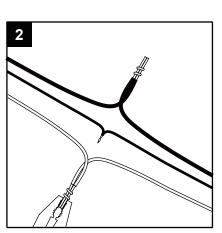
3. Attach wire nuts (BB). Tape wire nuts (BB) and wires together.
