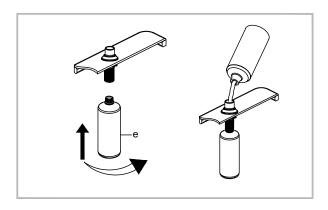
Reinsert pump (a) into dispenser base (b) from the top. Press the pump several times to make sure soap is evenly distributed.
