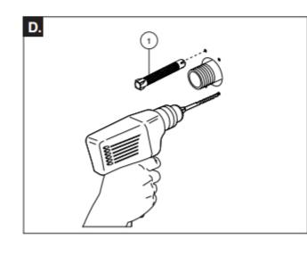
Connect to 1/2" IPS supply line. The pipe should extend 1/2" past the finished wall surface.
