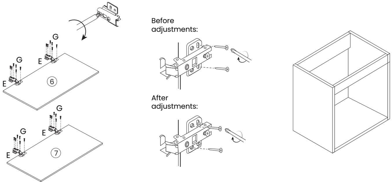
**Hinge/Door Adjustment and Realignment**
