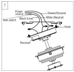
Make wiring connections using wire connectors provided as indicated above. White (Neutral) from house to White from remote receiver marked AC N. Black (Live) from house to Black from remote marked AC L. Connect all green grounded wires to Grounded wire from House. Make sure that no filaments are outside of the wire connector.
