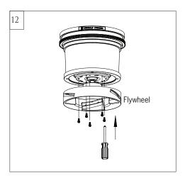
Insatll flywheel. Align the holes on flywheel with the screw holes on motor and install it onto the motor with set screws provided. tighten all screws securely.
