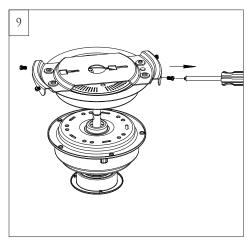
Loosen 2 screws across from each other and remove the other 2 preassembled screws from side of mounting plate (corresponding to installation step 10). Save screws for later use.
