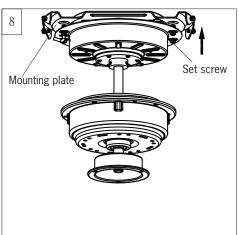
Lift motor assembly, aligning the set screws on the plate on top of motor with the screw holes on mounting plate. Tighten all screws securely.
