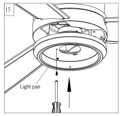
Place the lead wires from fan over the central hole of light pan
