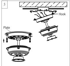
Use the set screws removed on the step 4 and fully install them onto the plate on top of motor.
