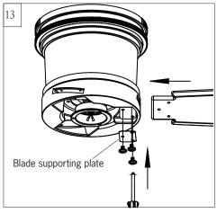
Insert blade into the slot on flywheel. Install blade with a blade supporting plate by the screws and washers provided, aligning each of the holes as shown and tighten all screws securely. Repeat this process for remaining blades.
