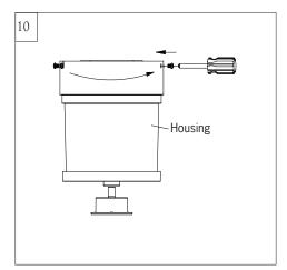
Attach housing onto mounting plate, aligning the keyhole slots on the housing with the screws on mounting plate and twist clockwise till tight. Reinstall the screw removed in step 9. Tighten all screws securely.
