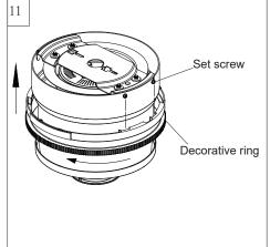
Attach decorative ring by locating the head of set screws on housing with grooves in the decorative ring and twist clockwise till tight.
