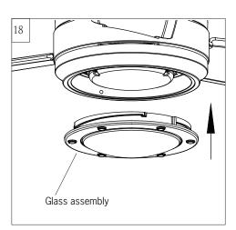
Attach glass assembly by locating dimples in light pan with grooves on the glass assembly and twist clockwise until tight.
