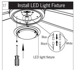
Connect white wire from fan to white wire from LED light fixture and then connect blue (or black) wire from fan to black (or blue) wire from LED light fixture. Be sure plugs connection clasped together completely. Attach LED light fixture onto the light pan, aligning the keyhole slots on the LED light fixture with the preassembled screws on the light pan. Twist clockwise till lock. Reinstall the screw removed in installation step 16. Tighten all screws securely.
