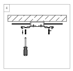
Remove 4 preassembled set screws from mounting plate. Save screws for later use.
