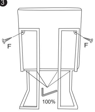
Using Self-Tapping Screw (F) lock 100%the frame and back
