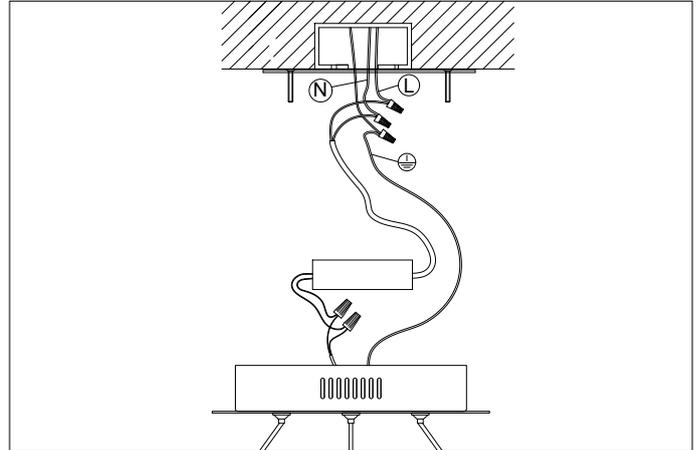
2. Place or hold the lamp in an elevated position in such a way that the wires can freely reach the ceiling junction box. Connect the 3 wires according to their colors. Black is the live wire, white is the neutral wire and brass wire is the earth wire.
