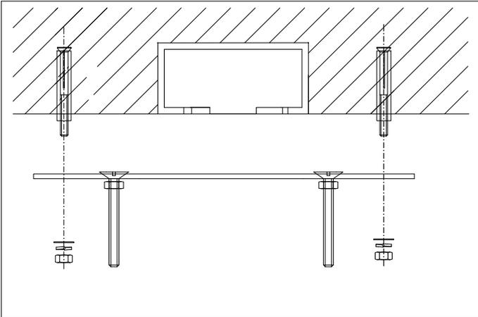
1. Fix the ceiling plate to the ceiling by using bolts and screws suitable to your ceiling type.
