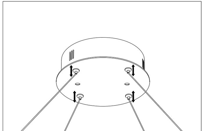
4. Adjust the length of the wires by pressing the wire lock on the ceiling canopy and pulling/pushing the wire through.
