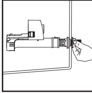
**Installing Fill Valve:** To install into tank, remove locknut and slide Fill Valve into the hole in tank. Next, position Fill valve to desired position and tighten the locknut.
