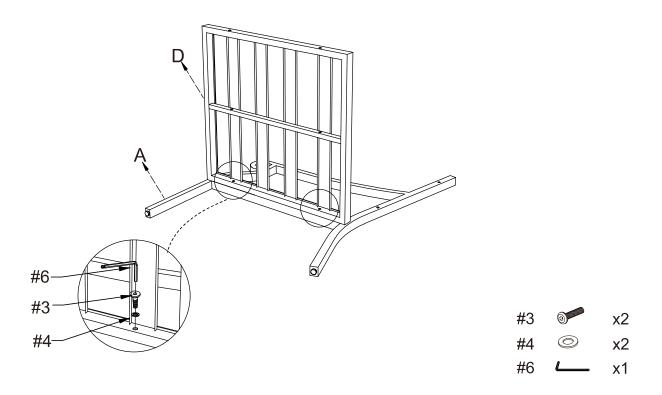
Step 2. Attach back panel (part C) to left arm panel (part A) and seat panel (part D) using long bolts (part #3), flat washers (part #4) and allen wrench (part #6).
