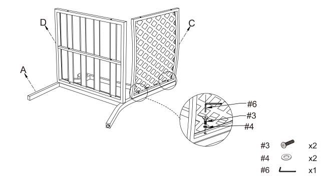
Step 3. Attach right arm panel (part B) to back panel (part C) and seat panel (part D) using long bolts (part #3), flat washers (part #4) and allen wrench (part #6).
