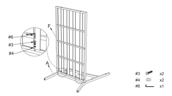
Step 6. Attach back panel (part E) to left arm panel (part A) and seat panel (part F) using long bolts (part #3), flat washers (part #4) and allen wrench (part #6).
