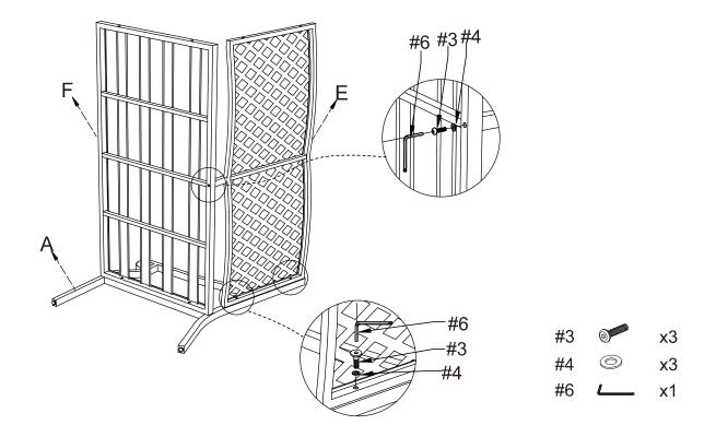
Step 7. Attach right arm panel (part B) to back panel (part E) and seat panel (part F) using long bolts (part #3), flat washers (part #4) and allen wrench (part #6).
