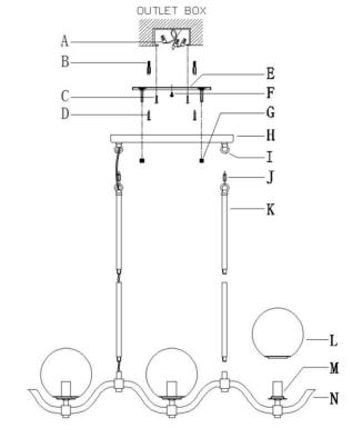
Step A1: According to your desired hanging height, choose and use the tubes (K). Carefully thread the fixture wires through the tubes (K), then screw the tubes (K) onto the iron frame (N).
