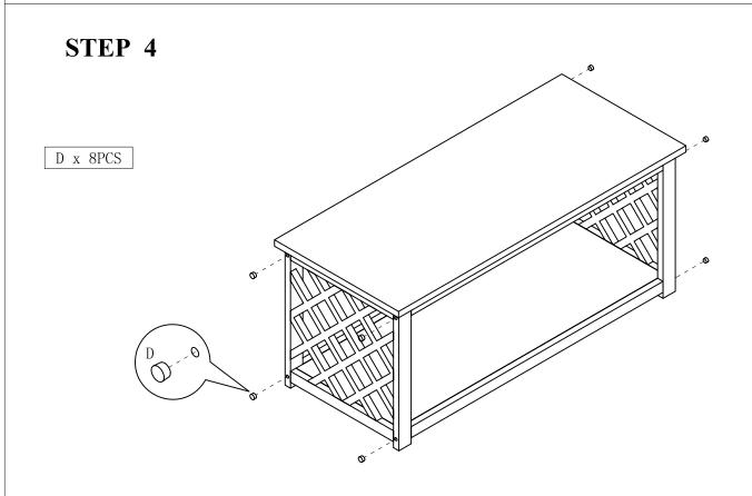
1. COVER HEX BOLT HOLE WITH WOOD PLUGS (D) AS SHOWN.
