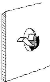
Wrap plumber tape around the pipe threads. It may be necessary to attach a pipe nipple (not included) to the supply line for your installation.
