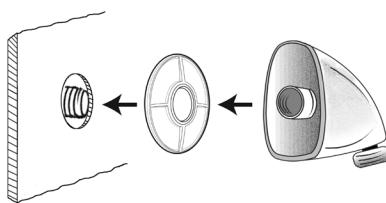
Apply a clean water sealant between the supply elbow gasket and the wall but DO NOT apply any sealant on the bottom part of the supply elbow; this will allow water to leak out, if needed. Secure the gasket around the pipe to assist in making a good seal between the supply elbow and shower wall. Fit the threads on the back of the supply elbow to the threads on the pipe and hand tighten until snug.
