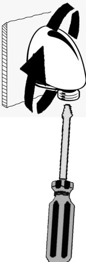
To fully tighten the supply elbow, insert a #2 phillips screwdriver into the outlet on the supply elbow, making sure the screwdriver reaches all the way into the supply elbow before tightening to avoid breaking the outlet. Tighten until the elbow is firmly against the wall and the threaded outlet is facing straight down. Make sure not to over-tighten where by the gasket is out of round.
