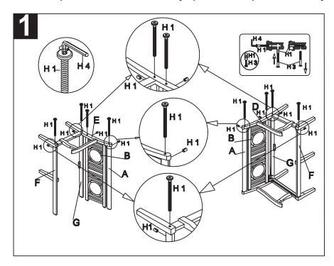
Step 1: attach right side (E) to the top (A) and back (B). Then attach support S (G) and support L (F) to the right side (E) as shown on the picture by using the Allen Bolt (H1) and tighten with the Allen Key (H4). Continue with the left side (D) in the same way. Make sure to tighten all bolts (H1) before you continue with step 2.
