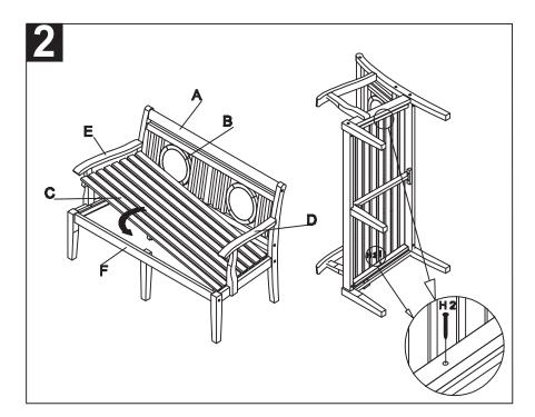
Step 2: put the seat (C) inside the bench as shown on the picture and use the screws (H2) to attach it to the bench by using a screwdriver.
