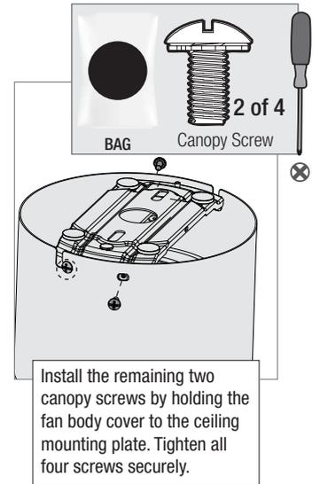
Install the remaining two canopy screws by holding the fan body cover to the ceiling mounting plate. Tighten all four screws securely.
