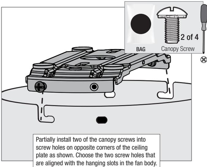
Partially install two of the canopy screws into screw holes on opposite corners of the ceiling plate as shown. Choose the two screw holes that are aligned with the hanging slots in the fan body.
