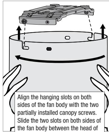
Align the hanging slots on both sides of the fan body with the two partially installed canopy screws. Slide the two slots on both sides of the fan body between the head of the screws and rotate the fan body counter clockwise so the screws hold the fan body firmly in place.
