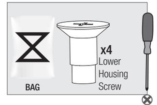
There are four holes on the motor. Lift the lower housing with the holes of the motor and align the grommet holes in the lower housing with the holes of the motor. It does not matter which hole you choose. Install the lower housing screws found in the hardware bag
