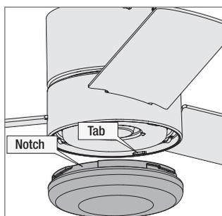
Lift the globe and align the notches in the globe with the tabs in the light kit.
