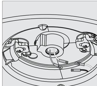
Connect the single-pin connectors from the LED assembly to the connectors from the fan. Connect the white wires together. Connect the blue and black wires together. Tuck the excess wiring above the LED assembly or feed back into the lower switch housing.
