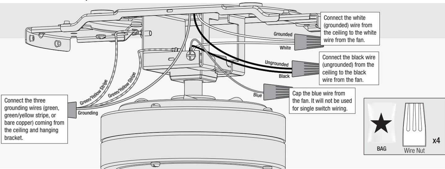
**! WARNING** The ceiling fan must be grounded. If the ground wire for the installation site is not present, immediately **STOP** installation and consult a qualified electrician.
