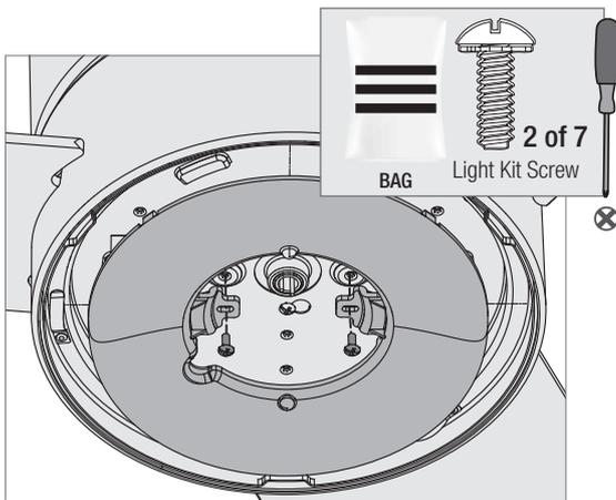
Raise the LED assembly to the trim ring. Align the screw holes in the LED assembly with the screw holes in the trim ring. Screw two light kit assembly screws, found in the hardware bag, through the LED assembly and into the trim ring.
