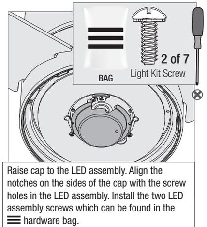
Raise cap to the LED assembly. Align the notches on the sides of the cap with the screw holes in the LED assembly. Install the two LED assembly screws which can be found in the hardware bag.
