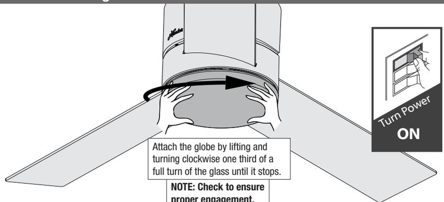
Attach the globe by lifting and turning clockwise one third of a full turn of the glass until it stops.
