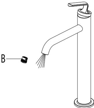
After installing faucet, remove aerator (B) with a coin. Turn water on for 30 seconds to remove any debris. Reassemble aerator (B).
