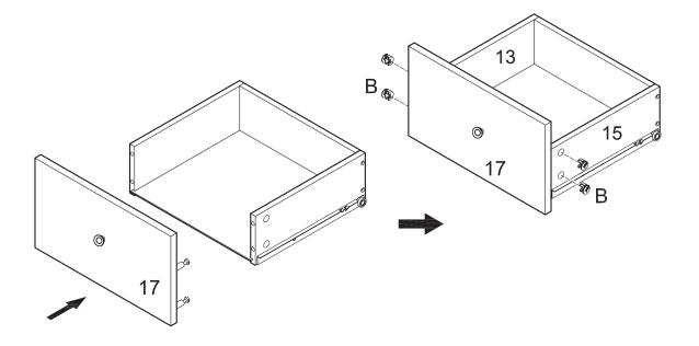
Attach drawer front (17) to the first drawer assembly using cam bolts as guides. Insert small cam locks (B) into drawer sides (13,15) and tighten with a screwdriver.
