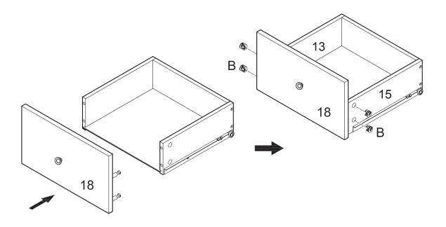
Attach drawer front (18) to the second drawer assembly using cam bolts as guides. Insert small cam locks (B) into drawer sides (13,15) and tighten with a screwdriver.
