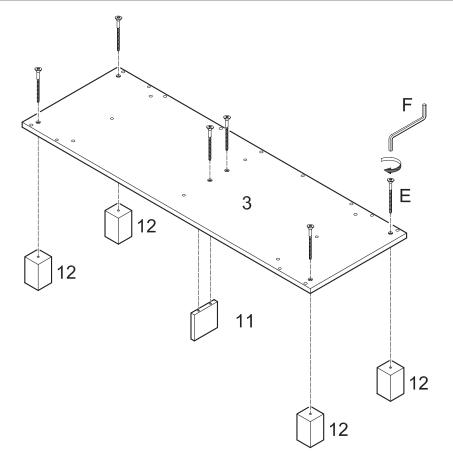
Attach feet (12) and stand support (11) to stand base (3) using large bolts (E) and wrench (F).
