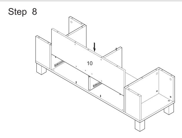
Carefully slide back panel (10) into place at the back of the stand assembly. Use cam bolts and dowels as guides.
