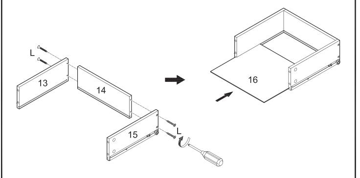
Attach drawer sides (13,15) to drawer back (14) using screws (L). Slide drawer bottom (16) into place along the grooves of the drawer assembly. Repeat this step for the second drawer.
