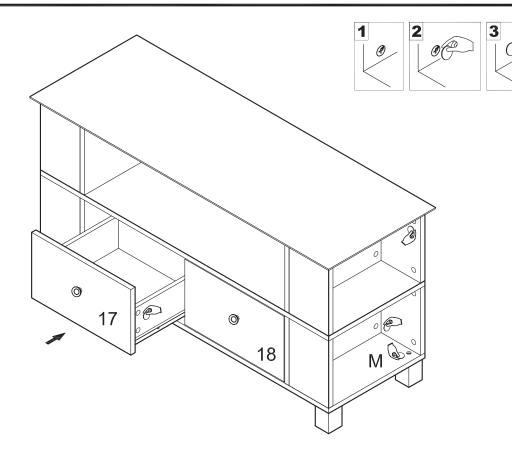
Carefully slide drawers into the stand assembly. Cover all visible cam locks with stickers (M) as desired.
