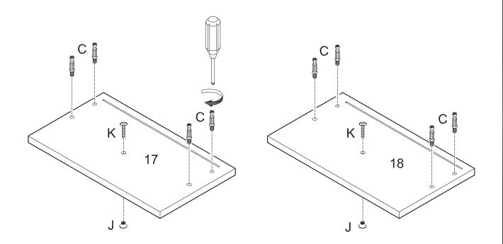
Screw short cam bolts (C) into drawer fronts (17,18). Attach handles (J) to drawer fronts (17,18) using small bolts (K).
