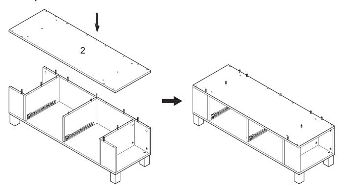
Carefully slide middle panel (2) into place on stand assembly. Use dowels as guides.
