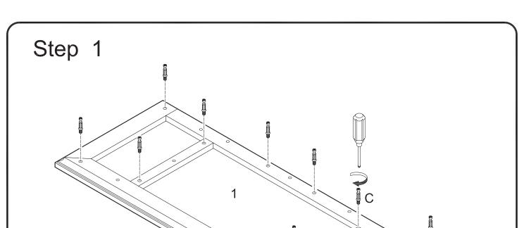
Screw short cam bolts (C) into stand top (1).
