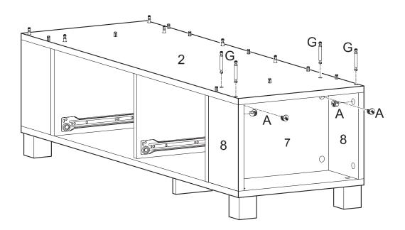
On opposite end of stand assembly, insert long cam bolts (G) into middle panel (2). Insert large cam locks (A) into panels (7,8) and tighten with a screwdriver.
