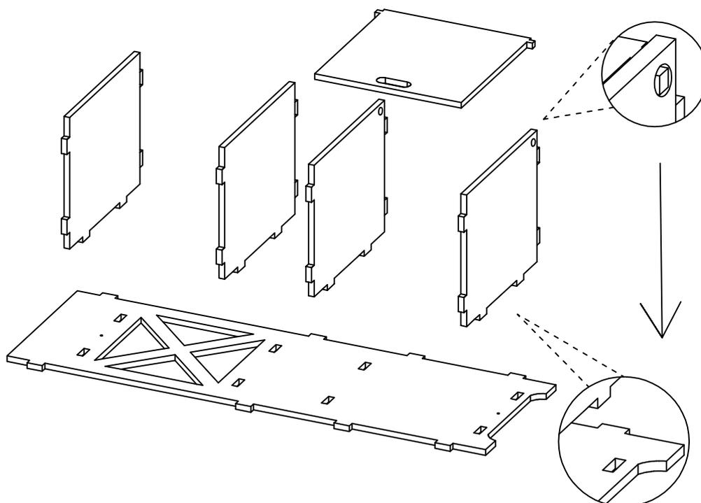
Attach the shelves to the back panel, by inserting them into the pre-drilled slats as shown above.
