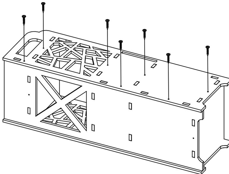
Insert and tighten left side panel with provided screws into pre-drilled holes to secure unit, as shown above.
