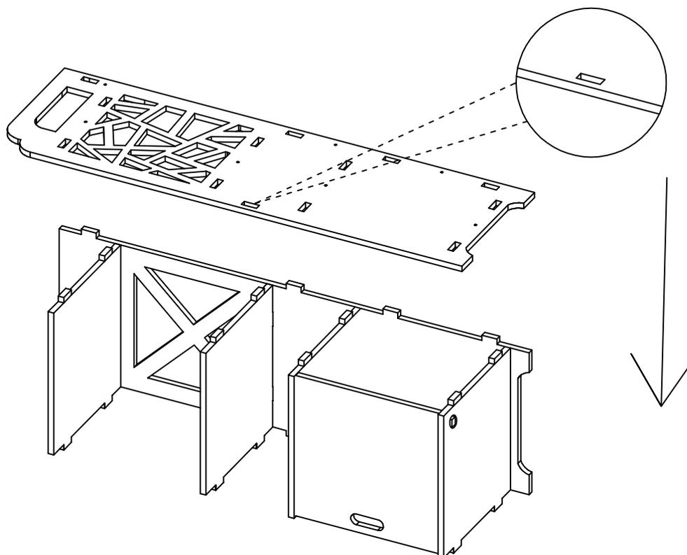
Attach the shelves to the right side panel, by inserting them into the pre-drilled slats as shown above.
