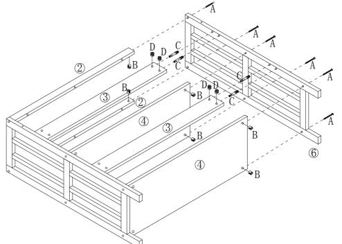
Make sure threaded hole of lock nut (B) faces direction of bolt (A) entrance hole.
