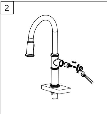
Step 2: Unscrew the locking nut with an adjustable wrench. Remove the ceramic disc cartridge.
