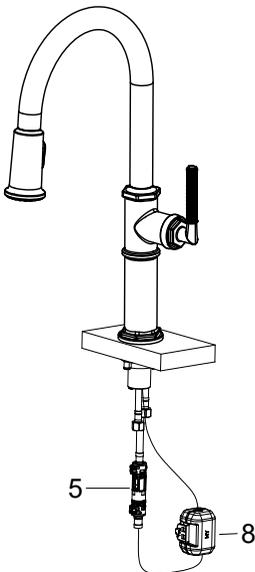
Connect the spray hose (9) to quick connector outlet (5) attached to the supply line. Install the weight (8) on the spray hose where it is marked.
