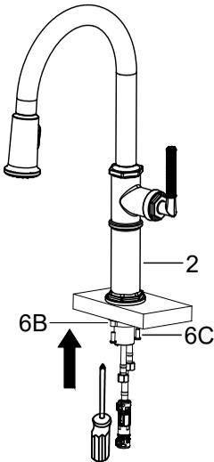
Adjust direction of faucet body (2) so that handle is on right side of faucet. Tighten mounting nut (6B) until snug. Tighten mounting screws (6C) to nut with Phillips screwdriver until snug.
