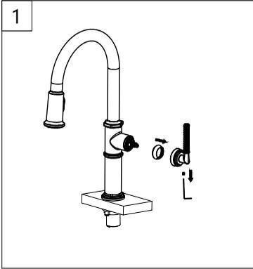
Step 1: Loosen the set screw with a hex wrench. Remove the handle and unscrew the cartridge cover by hand.
