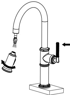
Remove spray head (1) from spray hose. Hold tip of spray hose. Turn faucet on and let the water run for 60 seconds to flush any debris.
