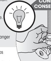
Firmly hand tighten the hose to the valve and add a quarter-turn using the proper wrench. Tighten more if needed.
