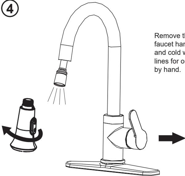
Remove the shower by hand. Turn the faucet handle all the way on, turn on hot and cold water supply and flush water lines for one minute. Reinstall shower by hand.
