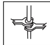
Tighten connection with two wrenches to prevent damage to tube body. Be careful not to bend the stem as this will void the product warranty.
