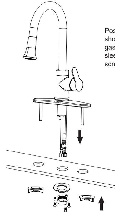
Position the faucet in order on the counter top as shown. **Don't forget the O-ring.** Assemble gasket assembly and lock nut to faucet threaded sleeve by hand and tighten the screws with screwdriver.
