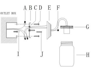
carefully tuck all wires into the outlet box .
