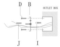
4. Attach the mounting plate assembly(B) to outlet box with mounting screws (D), plastic wall anchors (I) and wood screws (J).
