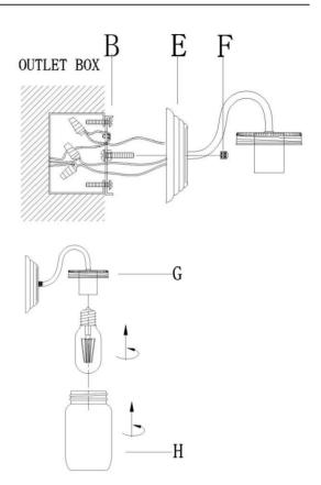
Install bulbs (Not included. Please do not exceed the maximum capacity recommended on the socket.)
