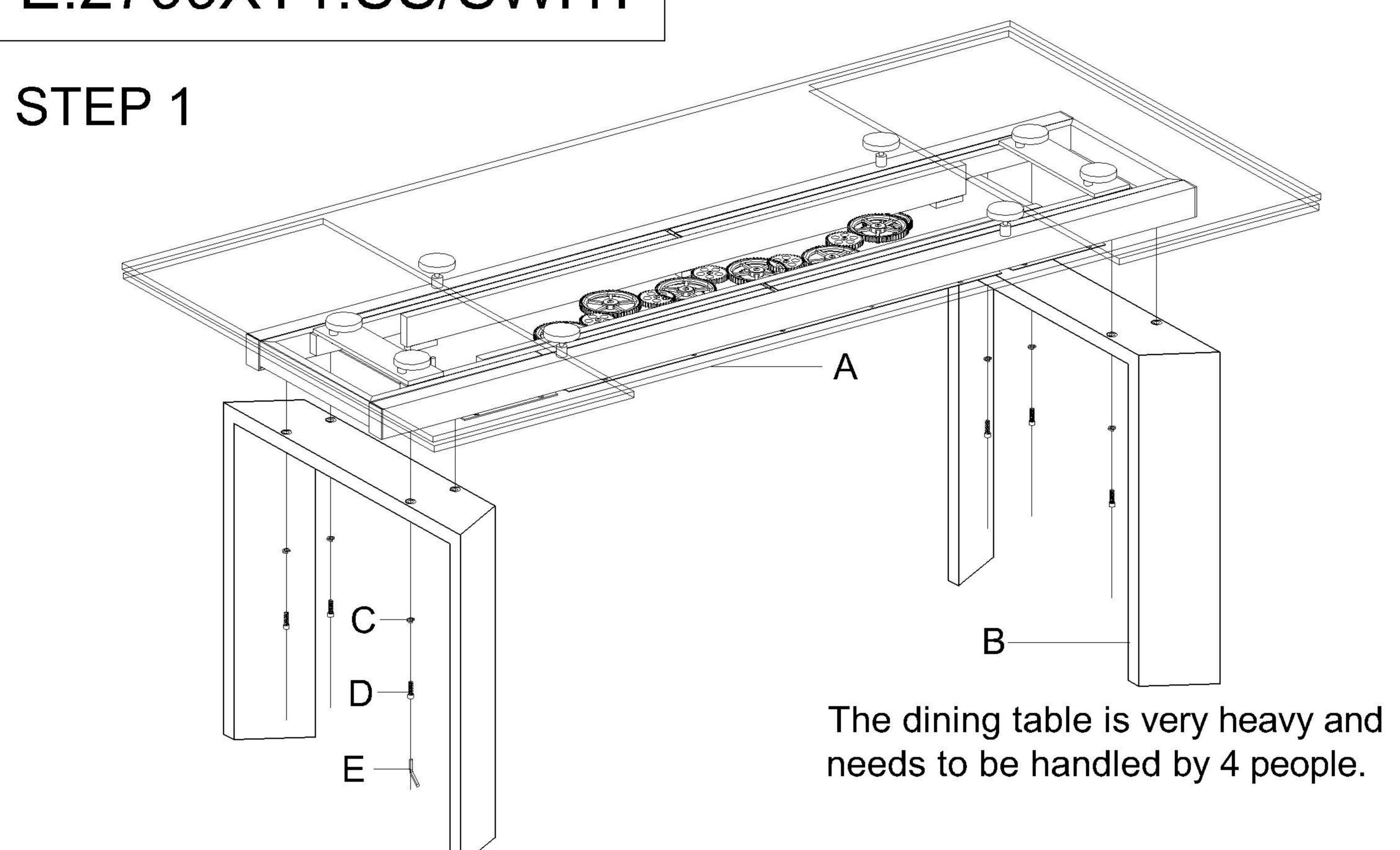
Warning! Table must be assembled right side up and not turned upside down or on its side. Doing so may damage the mechanism.
