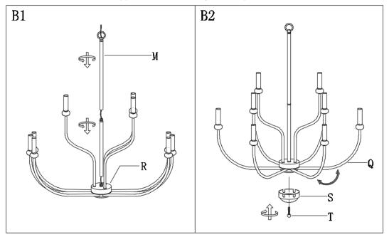
Step B1:Carefully thread stem(M) onto the top of wire house (R) until snug.
