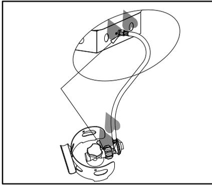
1. Make 2-3 oz. of leak check solution (one part liquid dishwashing detergent and three parts water).
