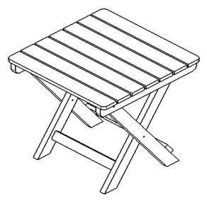
STEP 2: Use bolts (4) to attach leg (1) and (2) to the tabletop (3).
