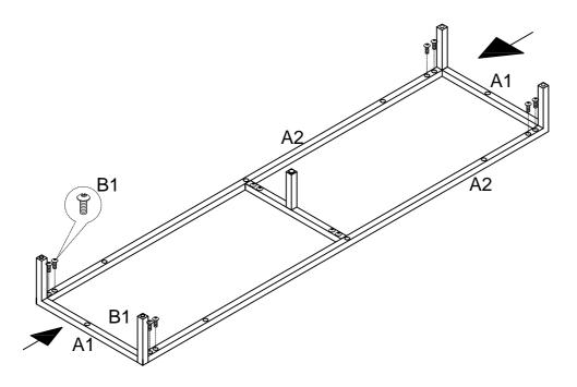
Insert and tighten Side Frames A1 to Rails A2 using Short Bolts B1. Note:Please do not tighten Bolts B1 unit Step 7.
