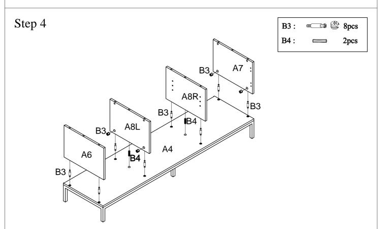
Assemble Side Panels A6&A7, Dividers A8(L&R) to Bottom Panel A4 using Cambolts&Camlocks B3 and Wood Dowels B4 as shown above.
