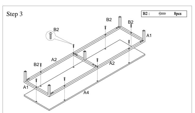
Assemble Side Frames A1,Rails A2 and Connect Bar with adjustable leg A3 to Bottom Panel A4 using Long Bolts B2.
