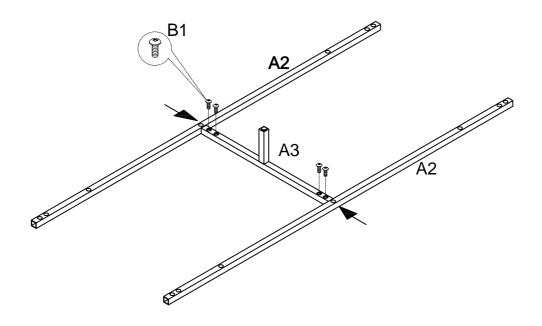
Insert and tighten Rails A2 into Connect Bars with adjustable leg A3 using Short Bolts B1. Note:Please do not tighten Bolts B1 until Step 7.
