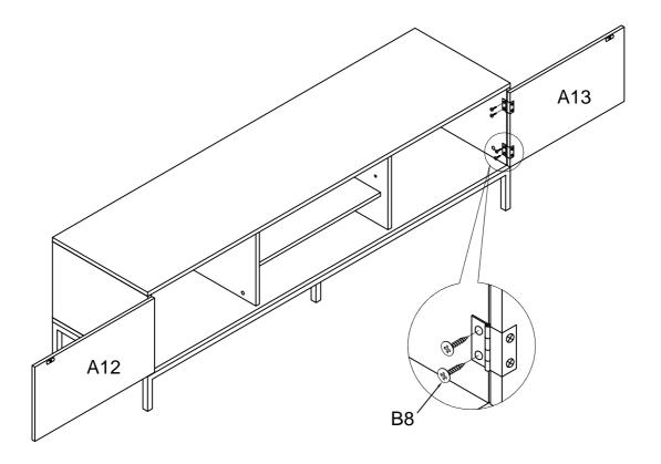
Attach Doors A12&A13 to Side Panels A6&A7 (L&R) using Screws B8. Note:Place this unit on the floor to check if it is stable before tightening all Bolts B1.
